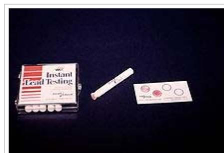
Testing kits are commercially available for detecting lead. These swabs, when wiped on a surface, turn pink in the presence of lead.
