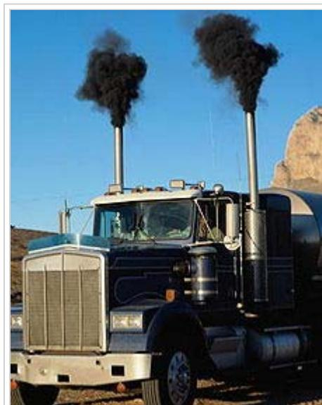
Emission of soot from a large diesel truck, without particle filters.
